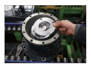
(26) After spreading loctite #242, assemble the bolt (7) (4 pcs).
