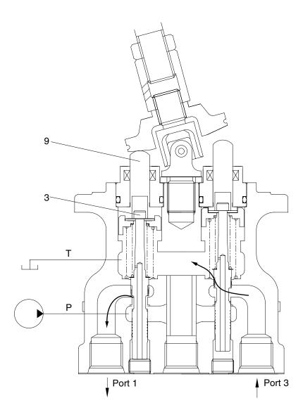
When the push rod (9) is stroked, the spool (3) moves downwards.
