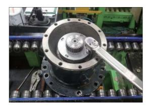
(27) Press parallel pin (31) by using press machine.
