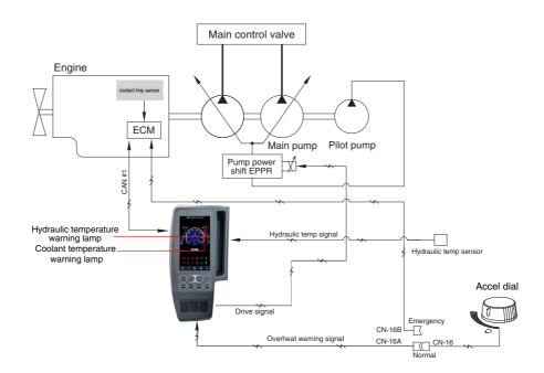
1. If the engine coolant temperature or the hydraulic oil temperature is overheated over 105°C, the warning lamp is ON and the pump input torque or the engine speed is reduced as below logic table.
