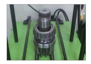
(22) Disassemble taper roller bearing (3) and oil seal (27) by using a press machine.
