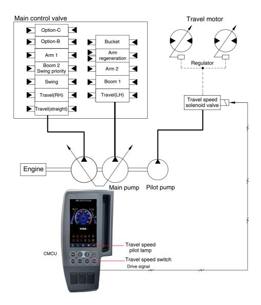
Travel speed can be switched manually by pressing the travel speed switch on the cluster.
