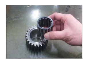
(18) Separate ring gear (1) from casing (8).
