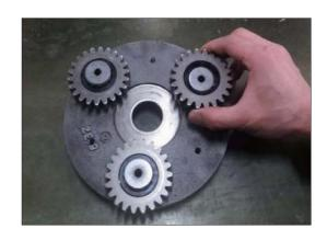
(7) Disassemble thrust plate (24).
