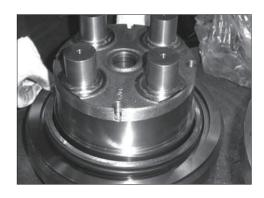
(12) Remove the oil seal (32) from spindle (101).
