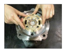
(7) Remove O-ring (19) from valve casing.
