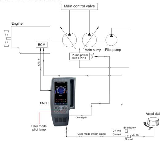
1) High idle rpm, low idle rpm and EPPR pressure can be adjusted and memorized in the U-mode.
