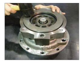
(15) Put spring (21) (22ea) in each hole of brake piston.
