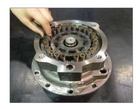
(16) Assemble plug (27) using 6 mm hexagon wrench.
