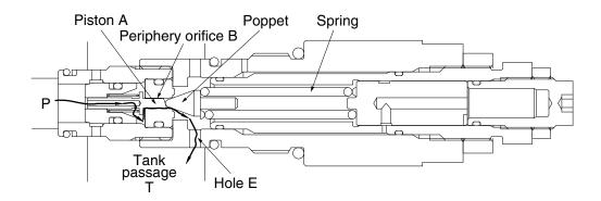
(3) Opening the poppet causes the pressure in chamber A to fall and the plunger to open. As the result the pressurized oil at port P runs into tank passage (T).
