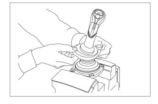
\*\* For valve with switch, remove cord also through hole of casing.
