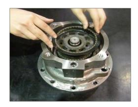
(12) Put separate plate (16) in casing.
