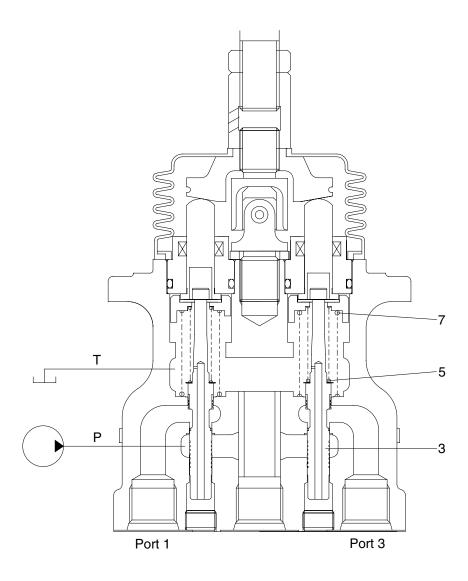
The force of the spring (5) that determines the output pressure of the pilot valve is not applied to the spool (3). Therefore, the spool is pushed up by the spring (7) to the position of port (1, 3) in the operation explanation drawing. Then, since the output port is connected to tank port T only, the output port pressure becomes equal to tank pressure.
