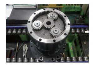
(2) Disassemble sun gear No.1 (22).
