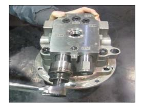
(26) Assemble snap ring (40) in shaft by using snap ring plier.
