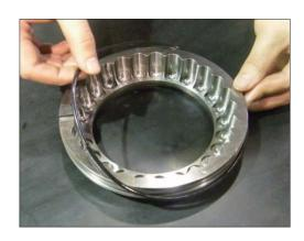
(14) Assemble parking piston (20) in casing using jig.
