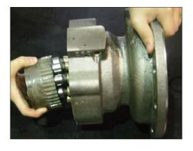
(11) Put friction plate (17) in casing.
