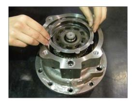
(13) Assemble O-ring (19) in brake piston (20).
