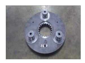
(2) After drilling  $\emptyset$  6 hole, assemble spring pin (15).(3 pcs)
