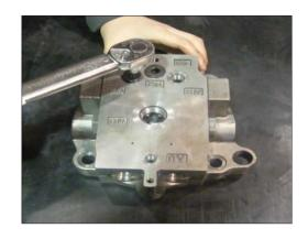
(17) Assemble reactonless valve assembly (39) in valve casing.
