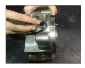
(21) Assemble spring pin (23) in valve casing using jig.
