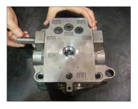
(18) Assemble plug (39-1) using hexagon wrench.
