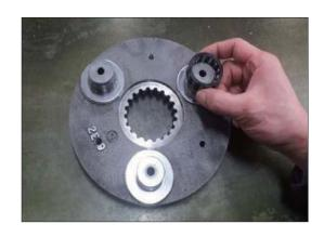
(9) Disassemble thrust washer No.1 (lower) (20). (3 pcs)
