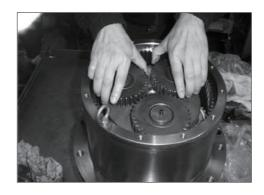
(9) Install drive gear (121) and thrust plate R (122) into the hub (105).
