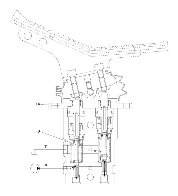
When the push rod (14) is stroked, the spool (8) moves downwards.
