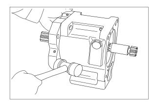
(11) Remove shoe plate (211) and swash plate (212) from pump casing (271).
