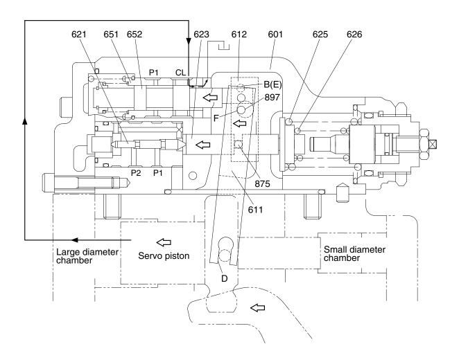
As the self pump delivery pressure P1 or the companion pump delivery pressure P2 decreases, the compensating rod (623) is pushed back by the action of the springs (625 & 626) to rotate lever 1 (612) around point E. Rotating of lever 1 causes the feedback lever (611) to rotate around the fulcrum of point D and then the spool (652) to move to the left. As a result, port CL opens a way to the tank port.
