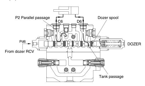
During the dozer down operation, the pilot pressure from the dozer control valve is supplied into the port Pc6 of the spring side and it shifts the dozer spool in the left direction.
