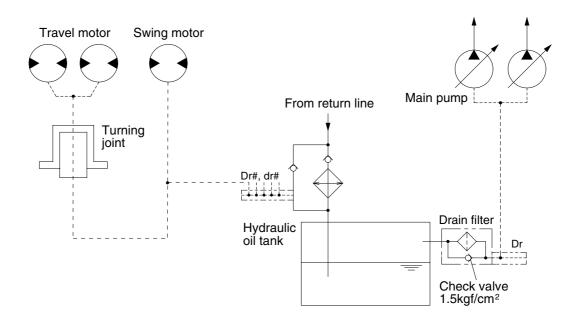
Besides internal leaks from the motors and main pump, the oil for lubrication circulates. These oil have to be fed to the hydraulic tank passing through drain filter.
