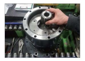
(32) Assemble carrier No.1 sub assembly.
