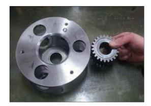
(14) Assemble carrier pin No.2 (14) to match the pin hole of the carrier No.2.(3 pcs)
