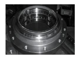
(4) Install the spindle (101) into the hub (105) assembly.
