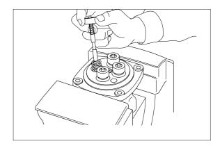
(5) Assemble O-ring (15) onto plug (14).
