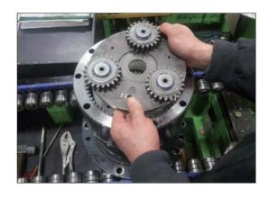
(33) Assemble sun gear No.1 (22) of which grinding surface is faced downward.
