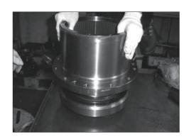
(10) Remove the floating seal (102), seal ring (129), angular bearings (125, 2EA), snap ring (106) and O-ring (130) from the hub (105).
