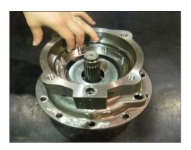
(6) Assemble cylinder spring (8) (9ea) in rotary block (6).
