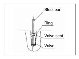
③ Remove the valve seat (18) by injecting compressed air from the access hole in the spindle (101) after caulking the hole of valve seat (18).
