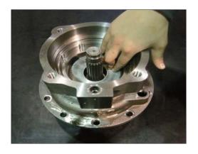
(5) After applying grease on O-ring (18), insert O-ring in casing (1).
