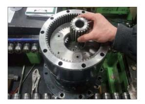
(12) Disassemble carrier No.2 sub assembly.
