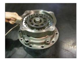
(13) Lay casing down horizontally and remove rotary block assembly from shaft. And remove all friction plate (17) and separate plate (16).
