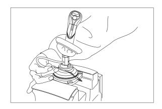
(4) Loosen lock nut (22) and adjusting nut (21) with spanners on them respectively, and take out handle section as one body.
