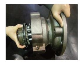
(14) Separate piston assembly (14, 15), trust ball (12), retainer plate (13).
