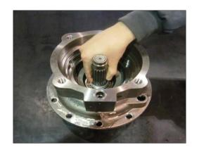
(18) Turn casing (1) upside down and remove oil seal (2) using jig.
