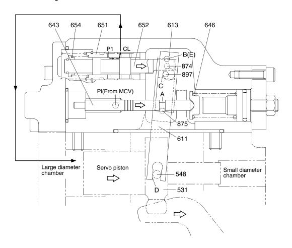
As the pilot pressure Pi rises, the pilot piston (643) moves to the right to a position where the force of the pilot spring (646) balances with the hydraulic force.
