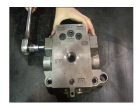
(9) Remove plug assy (27) (2ea) using 6 mm hexagon wrench.
