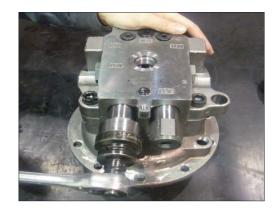
(5) Unscrew M16 socket bolt 33 (2EA), 34 (2EA) using 14 mm hexagon wrench.
