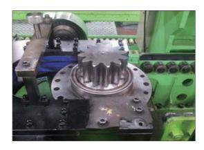
(23) After fixing drive shaft so that it does not fall, and then turn it over, press taper bearing (4).
