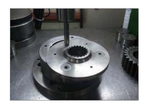
(11) Disassemble sun gear No.2 (16).
