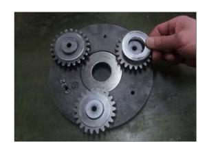
(6) Disassemble planetary gear No.1 (18).(3 pcs)
