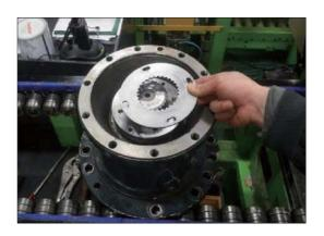
(20) Disassemble ring nut (5) by using the jig.
