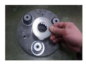
(8) Disassemble needle bearing No.1 (19). (3 pcs)
