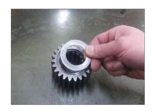
(12) Assemble thrust plate (24).
