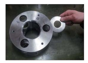
(16) Disassemble thrust washer No.2 (13).(6 pcs)
