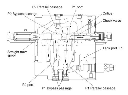
This function keeps straight travel in case of simultaneous operation of other actuators (boom, arm, bucket, swing) during a straight travel.
