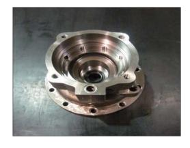
(2) Mount ball bearing (3, 24) on drive shaft (4) using shrink fitting method.
