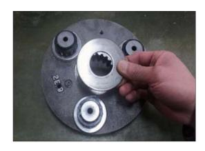
(7) Assemble planetary gear No.1 (18) of which groove is faced downward.(3 pcs)
