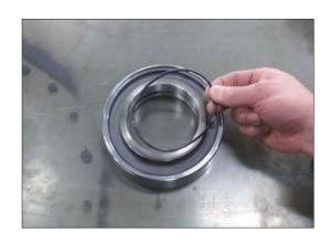
(24) Disassemble the outer ring of taper roller bearing (3) in casing (8) by using the jig.
