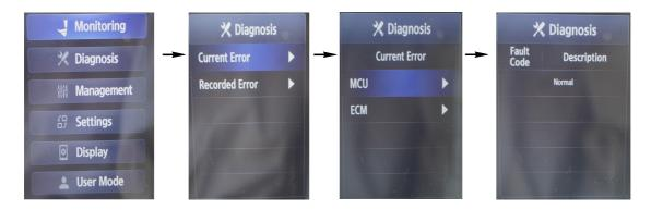
· The active faults of the CMCU can be checked by this menu.
