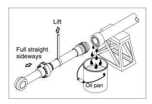
Note that the plated surface of rod assembly (2) is to be lifted. For this reason, do not use a wire sling and others that may damage it, but use a strong cloth belt or a rope.
