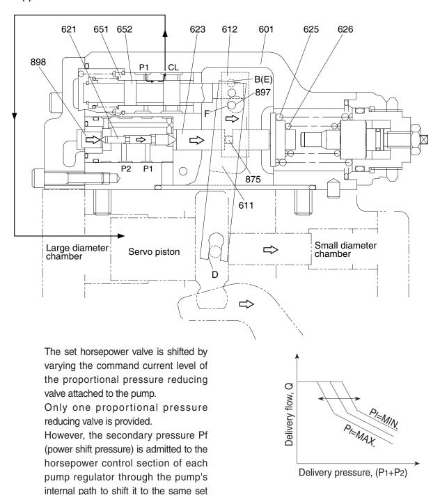
This function permits arbitrary setting of the pump output power, thereby providing the optimum power level according to the operating condition.
