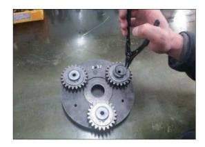
(5) Disassemble thrust washer No.1 (upper) (32).(3 pcs)
