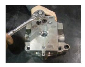
(10) Remove plug assy (30) using 17 mm socket wrench and separate spring; spring (29) and plunger (28). (same for the set on opposite side)
