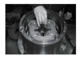
(6) Remove the thrust washer (109), planetary gears F (108), needle bearings (111) and collar (112) from hub (105).
