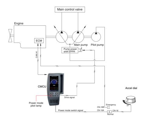
Mode selection system (micro computer based electro-hydraulic pump and engine mutual control system) optimizes the engine and pump performance.
