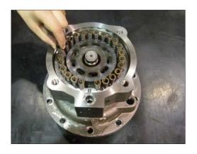
(12) Disassemble brake piston (20) from casing using air gun.
