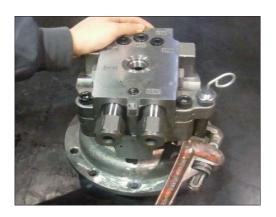
(4) Disassemble two sets of relief valve assembly (51) using socket wrench.
