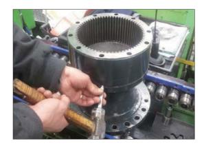
(19) Loosen bolt (7) (4 pcs), and disassemble lock plate (6).
