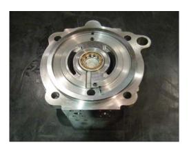
(8) Remove plug (39-1) using hexagon wrench and take out reactionless valve assembly (39). (same for the set on opposite side)
