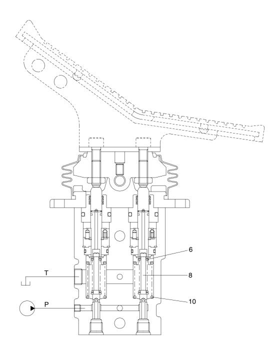
The force of the spring (6) that determines the output pressure of the pilot valve is not applied to the spool (8). Therefore, the spool is pushed up by the spring (10) to the position of port 2 in the operation explanation drawing. Then, since the output port is connected to tank port T only, the output port pressure becomes equal to tank pressure.
