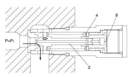
③ The oil flows into chamber (g) via orifice (m) and (n). When the pressure of chamber (g) reaches the preset force (FSP) of spring (4), the piston (7) moves left and stop the piston (7) hits the bottom of stopper (8).
