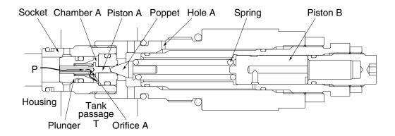
(2) When the pressure at (P) becomes equal to the set pressure of the spring the hydraulic oil passes through the piston (A) pushes open the poppet and flows to tank passage (T) through the plunger internal passage, periphery orifice A, chamber A, periphery orifice B and the hole (E).
