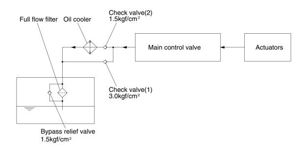
All oil from each actuator returns to the hydraulic tank through the control valve.
