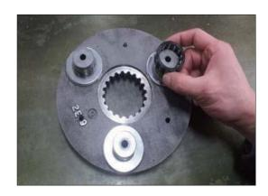
(6) Assemble thrust plate (24).
