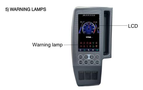
\* The warming lamp lights ON and the buzzer sounds when the machine has a problem. In this case, press the buzzer stop switch and buzzer stop, but the warming lamp lights until the problem is cleared.
