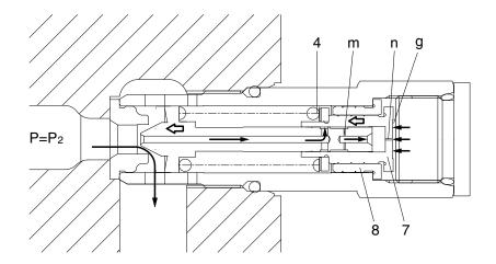
④ When piston (7) hits the bottom of stopper (8), it stops moving to the left any further. As the result, the pressure in chamber (g) equals (Ps).
