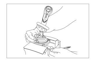
(18) Determine handle direction, tighten lock nut (22) to specified torque to fix handle.
