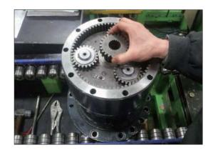
(3) Disassemble carrier No.1 sub assembly.
