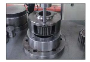
(14) Disassemble planetary gear No.2.(3 pcs)
