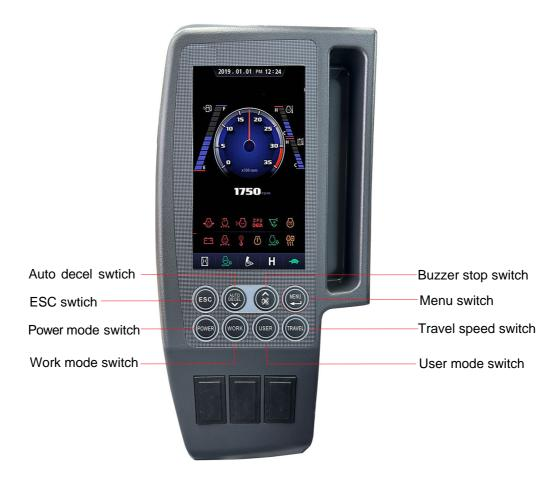
\* When the switches are selected, the pilot lamps are displayed on the LCD.
