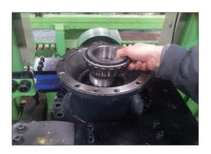
(24) Assemble nut ring (5) by using the jig.  $\divideontimes$  Tightening torque : 3.5  $\pm$  0.4 kgf  $\cdot$  m (25.3  $\pm$  2.9 lbf  $\cdot$  ft)
